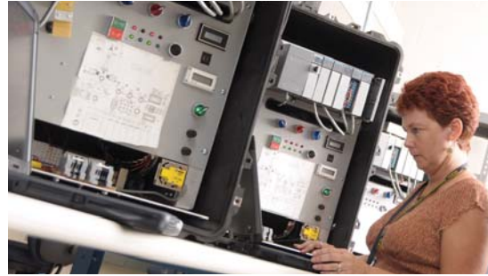
Allen Bradley SLC500 Mobile Units
